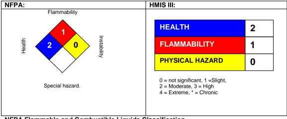
NFPA Flammable and Combustible Liquids Classification Combustible Liquid Class IIIB
